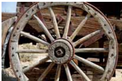
A wooden wagon wheel with a steel tyre for increased durability
