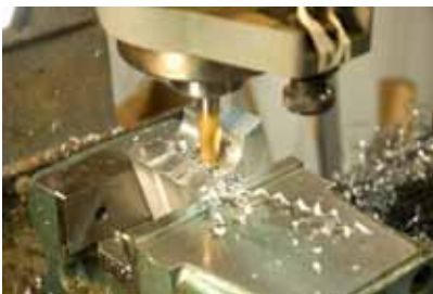
Machining aluminium and making swarf
