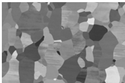
Figure 3.7—The grain structure within the metal
