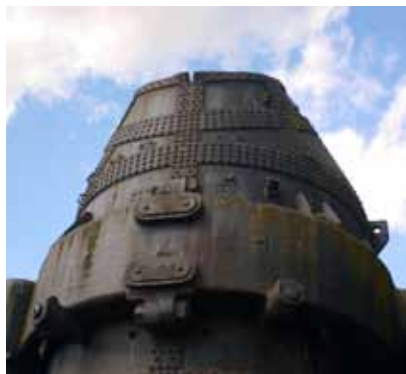
A Bessemer converter in which hot air is blown through liquid iron to burn off impurities and so produce cheap, malleable steel
