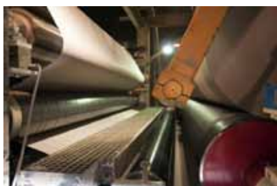
Dry end of a paper making machine
