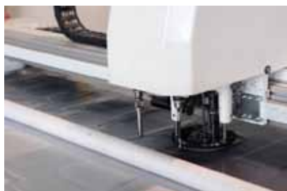
CNC machine cutting and perforating fabric
