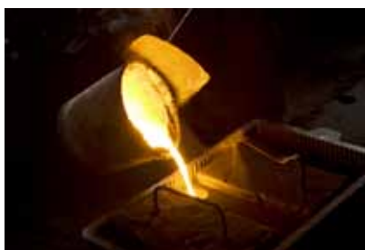
Direct casting of a steel part in a sand mould
