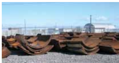
Recovered ship plate ready for re-rolling
